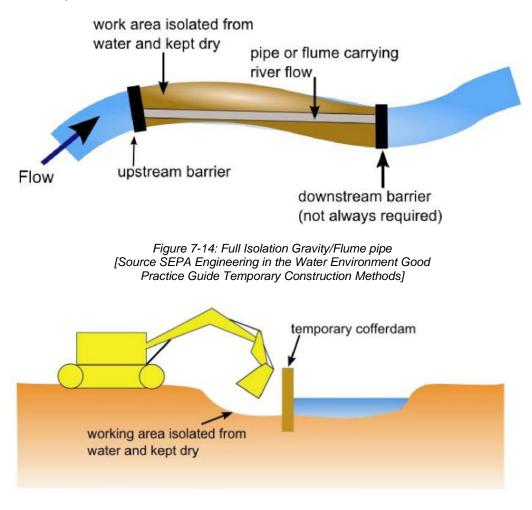
Figure 7-15: Partial Isolation Cofferdam [Source SEPA Engineering in the Water Environment Good Practice Guide Temporary Construction Methods]
