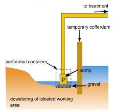
Figure 7-9 Submersible Pump on a gravel base and perforated container [Source SEPA Engineering in the Water Environment Good Practice Guide Temporary Construction Methods]
