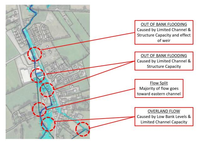
Figure 7-8 Flood Mechanisms – Overview
